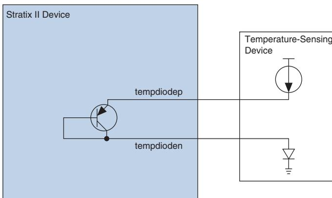
Table 3–6 shows the specifications for bias voltage and current of the Stratix II temperature sensing diode.
