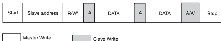
Figure 3. I 2 C Command Format
