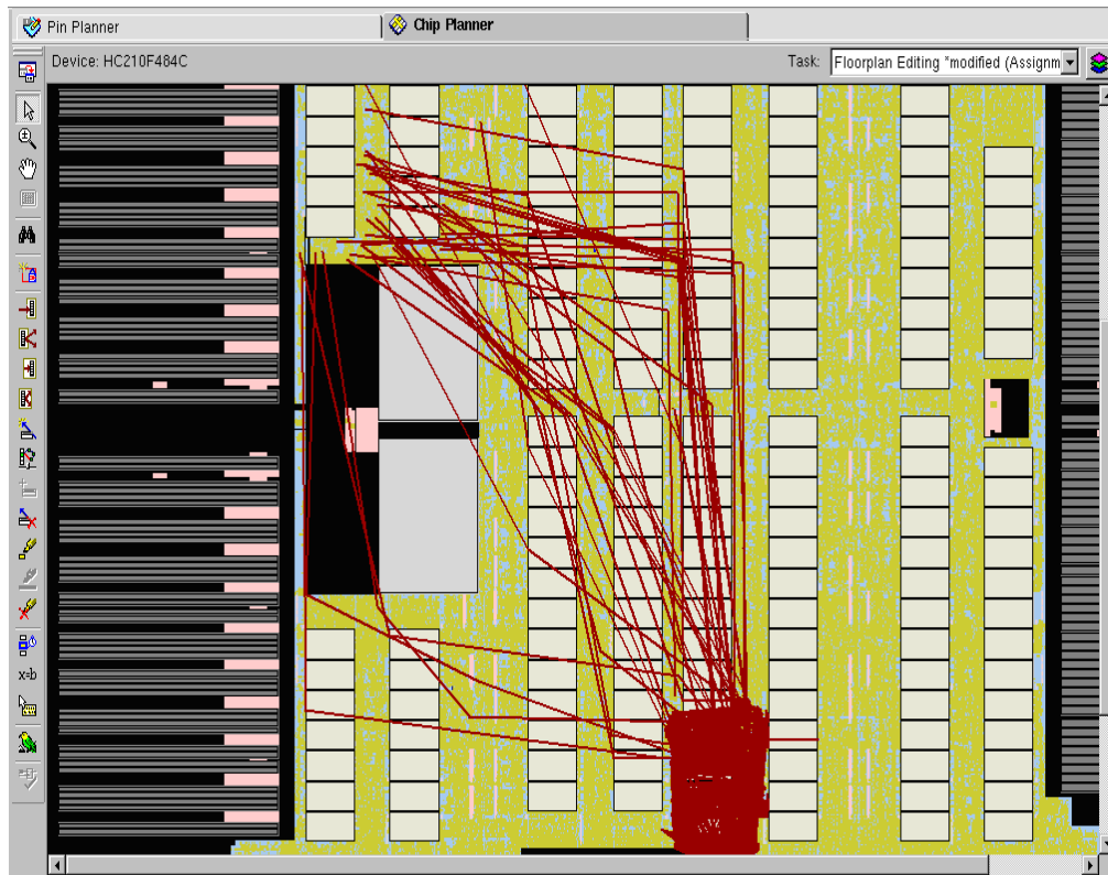
Figure 13. Example of a Poorly Placed Block, as Indicated by the Show Node Fan-In and Show Node Fan-Out Fly Lines
